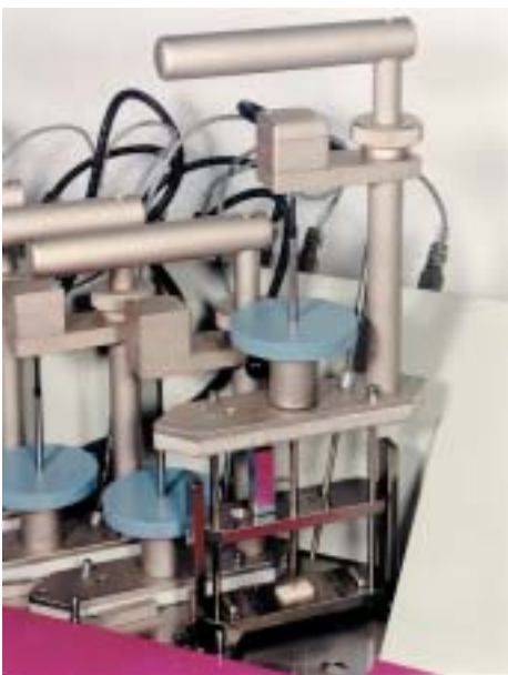
VICAT test station
